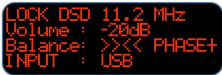
If no key is pressed within 10 seconds the *ZeroUno* DAC automatically stores the values shown at the display and switches back to the **PLAY/MUTE** mode.
