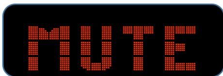
When the **MUTE** key is pressed, the *ZeroUno* DAC is muted and the display *never* goes back to the standard size view till the MUTE key is pressed again.
