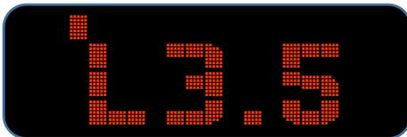
When the **BALANCE** keys are pressed, the balance changes in 0.5dB steps. Range is **LEFT** -5.0dB to **RIGHT** +5.0dB. To help the user the 1<sup>st</sup> row of the display reports a bar showing the position of the balance value in the range -5.0dB to 5.0dB.
