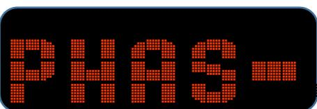
When the **LISTENING POLARITY** key is pressed the value is toggled between absolute polarity listening, showed PHASE+, and inverse absolute polarity listening, showed PHASE-.
