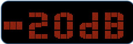
When the **VOLUME** keys are pressed, the attenuation changes with steps of 1.0dB. Range is -60dB to 0dB. If the key is kept pressed the attenuation changes quickly.
