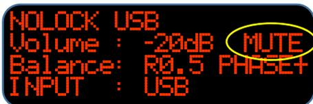
When a MUTE appears at the display in standard size means there is no signal locked at the selected INPUT and the *ZeroUno* DAC automatically forces to the MUTE condition. This function is totally independent from the MUTE imposed by the user.
